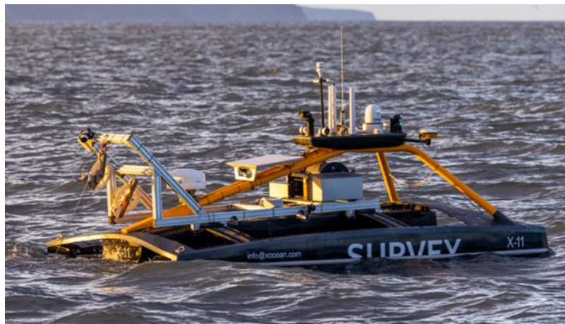
Figure 2: USV with hull mounted sensors
