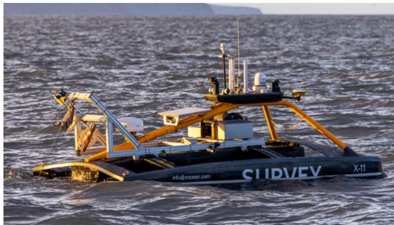
Figure 2: USV with hull mounted sensors
